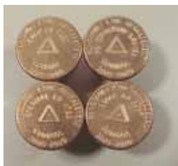
Special Monument caps for the retracement survey.
